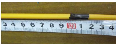
Pic 3: the length of stripped fiber cable
