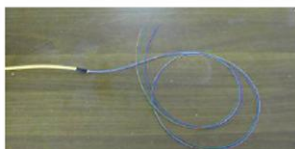
Pic4: fiber after stripping
